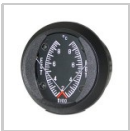
Double EGT (exhaust gas temp for 914)
