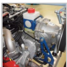
Slipping clutch in gear box for 914
